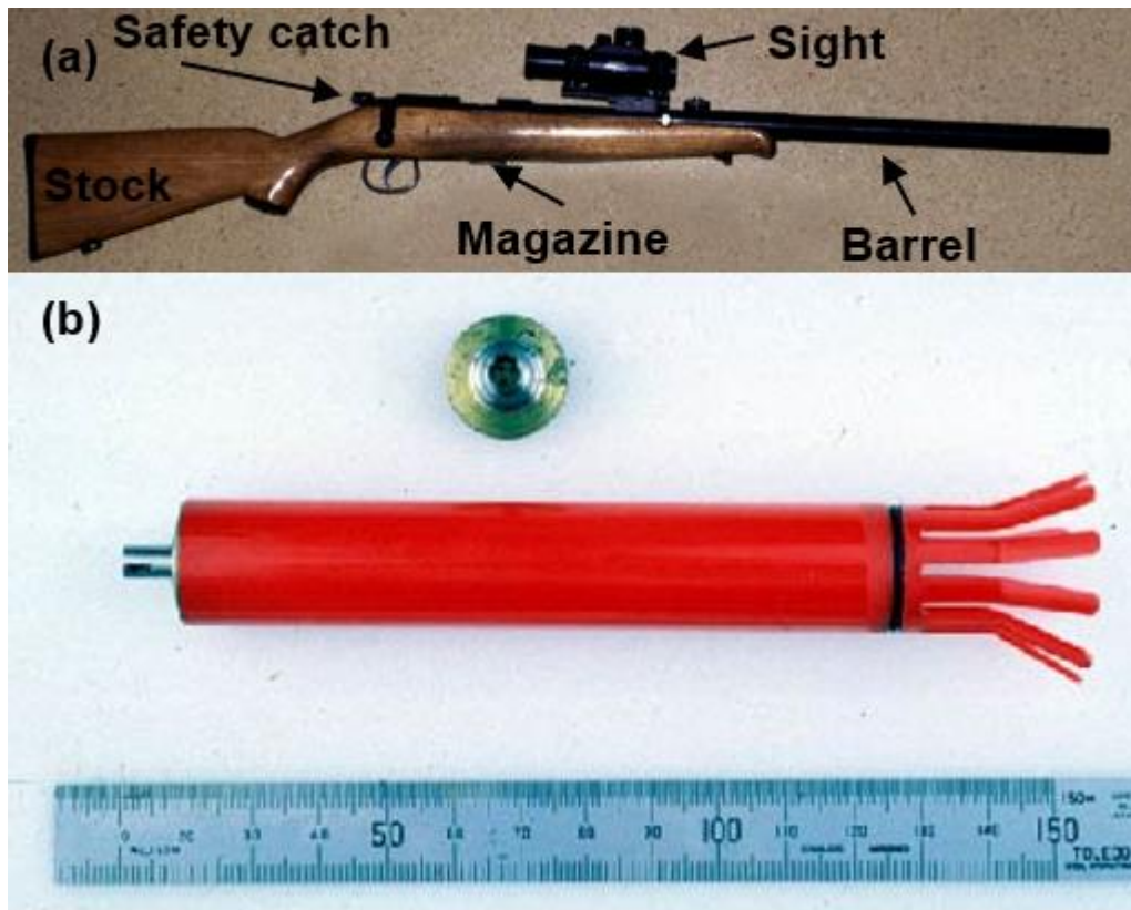
Figure 1 The PAXARMS biopsy system. (a) Assembled 0.22 caliber rifle with Pro-Point red-dot sight. (b) Biopsy dart and biopsy tip. Photos taken from Murdoch University Cetacean Research Unit.
