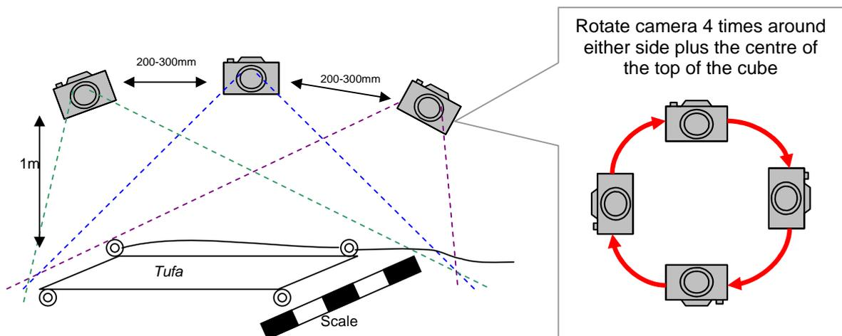
**Figure 4: Camera positioning for photographing a new tufa site.**
