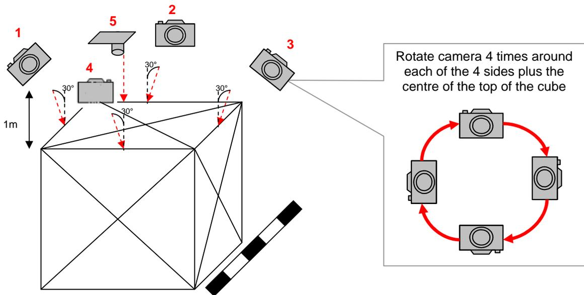
**Figure 1: Camera positioning for calibration.**
