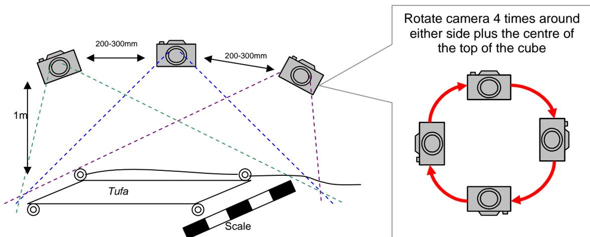
**Figure 2: Camera positioning for photographing established tufa sites.**
