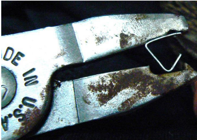
Figure 3 Set up of a metal ear tag in the pliers. Photo: Christine Freegard/DBCA.
