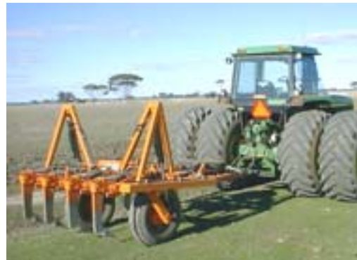
Figure 8. A seven tyned trailable implement with hydraulic tyne breakout.
