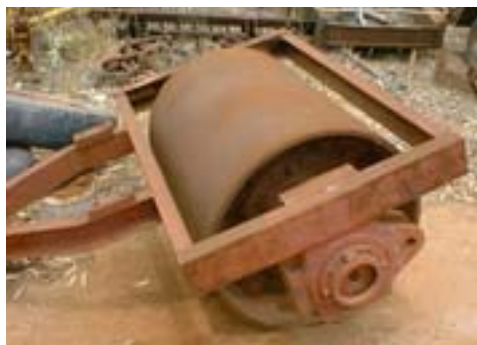
Figure 11. This roller was used successfully to shatter 'dry' clay boulders on the soil surface. It was also used for lowering (flattening and smoothing also) the profile of a mound (see mound ploughing section).
