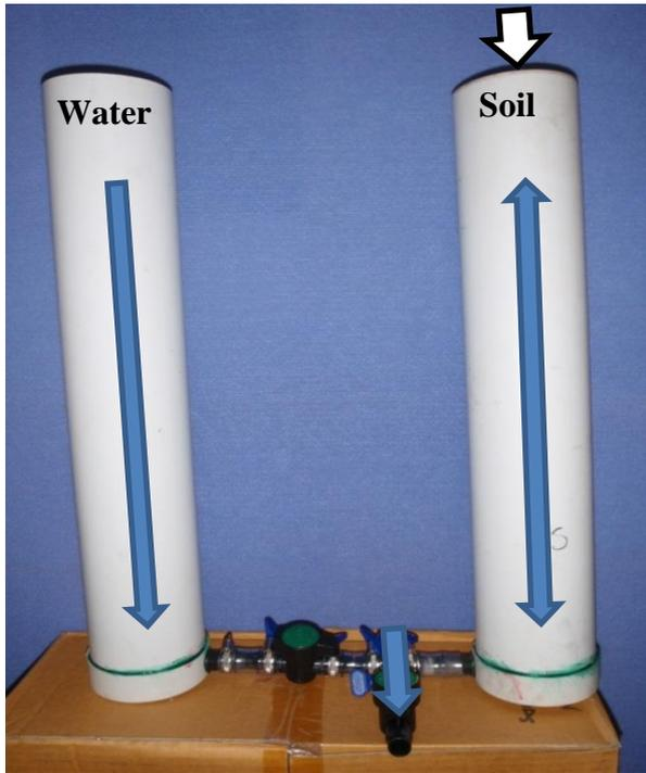
Figure 2- A photograph of the columns used, highlighting water movement from the water to soil column, which imitates the rise and fall of groundwater following rainfall
