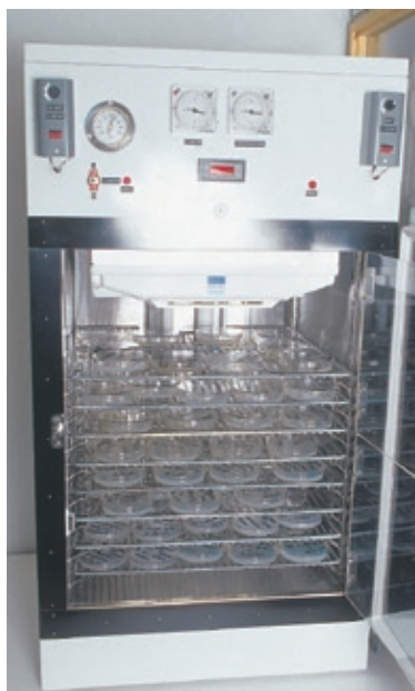
A temperature and light controlled incubation cabinet can be used to assess the germination capability of seed.
